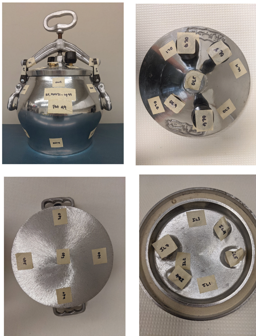
Fig. 1 Example XRF testing locations on an aluminum Afghan pressure cooker (Pot #49). Top left: Labeled pressure cooker body. Bottom left: Labeled base. Top right: Labeled outer surface of lid. Bottom right: Labeled inner surface of lid.
