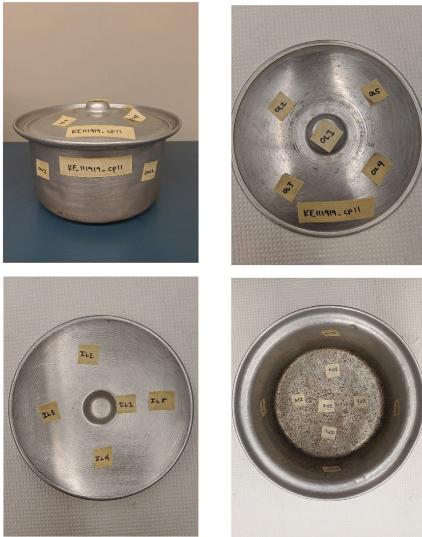
Fig. 2 Example XRF testing locations on a typical aluminum cookpot (Pot #11). Upper left: Labeled body of cookpot. Lower left: Labeled inner surface of lid. Upper right: Labeled outer surface of lid. Bottom right: Labeled inner surface of cookpot.
